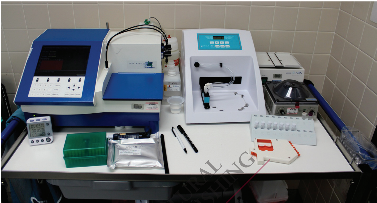
Figure 13-3. Mobile equipment for performing the PTH assay in the operating room.
